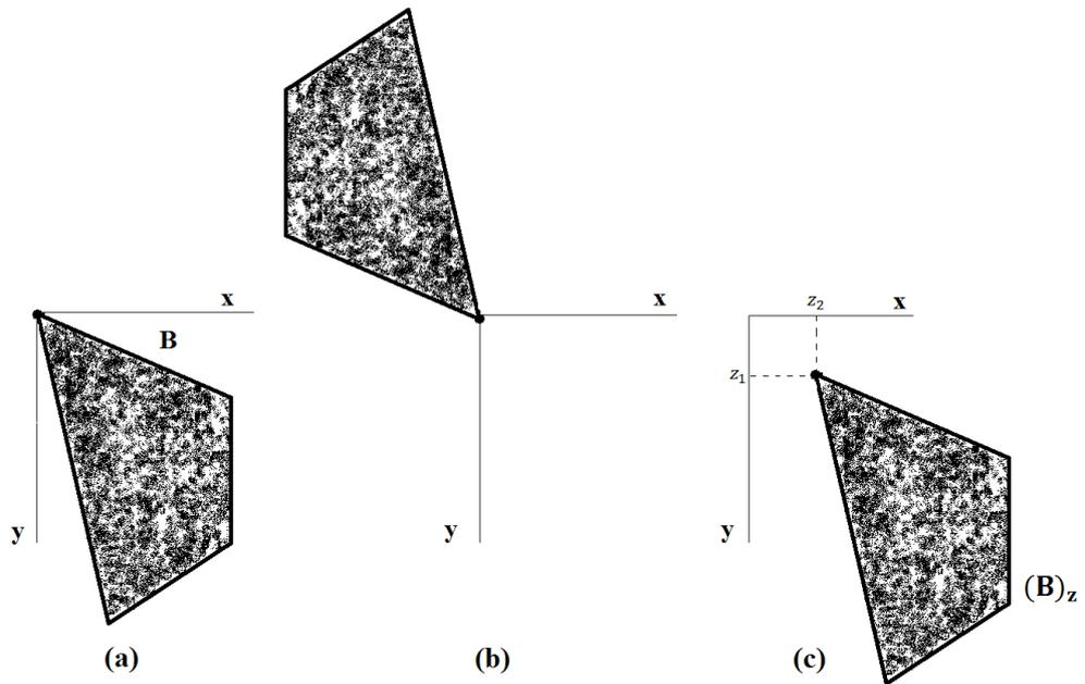
**Figure 2.2 (a) a set of B, (b) reflection of set B and (c) translation of set B by z**
