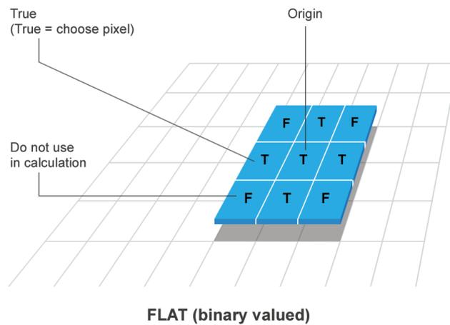
**Figure 2.8 Flat Structuring Elements**
