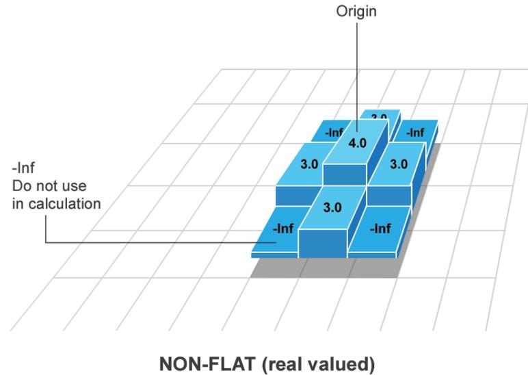
**Figure 2.9 Non-Flat Structuring Elements**
