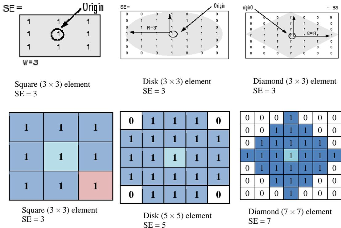
**Figure 2.11 Some Shapes of Structuring element**
