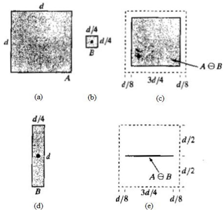
**Figure 2.4** (a) Set A. (b) Square structuring element, B (c) Erosion of A by B, shown shaded. (d) Elongated structuring element.(e) Erosion of A by B using (d).
