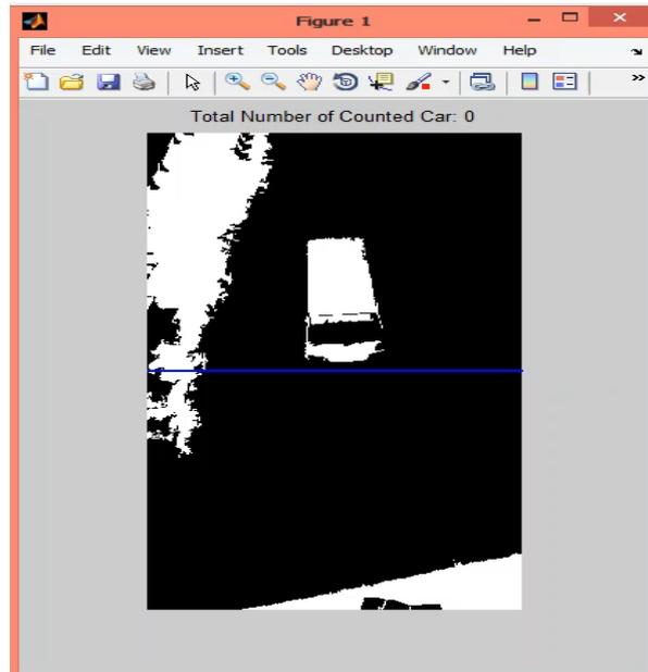
**Figure 4.6 Before the Object (Detected Car) Passing Through the Line, Count 0,**
