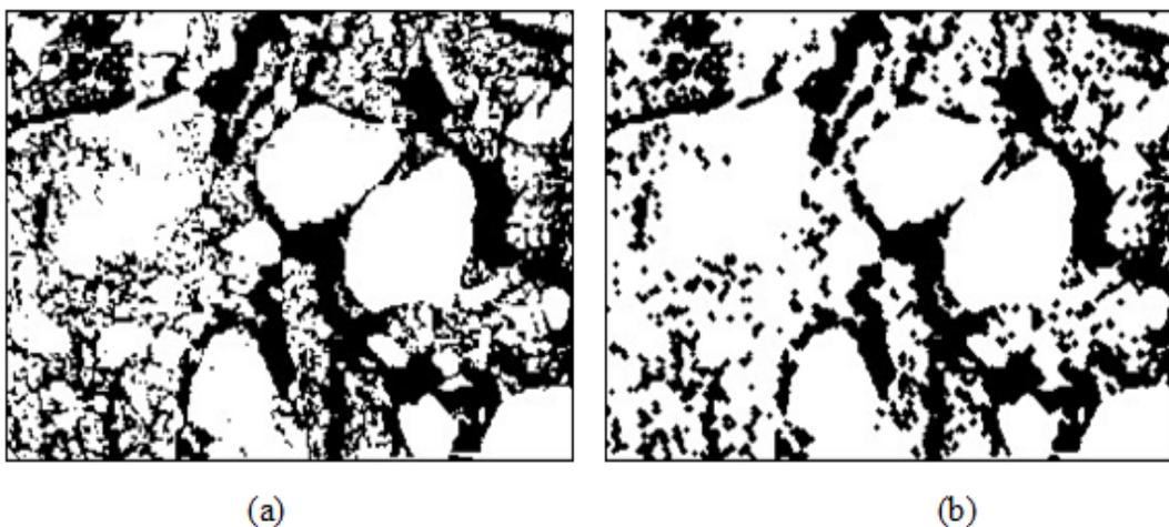
**Figure 2.1 (a) soil image subset (b) closing operation result of (a) using approximation a disc of radius 1.0**
