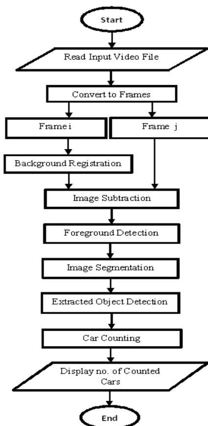
**Figure 4.1 System Flow Diagram of the Car Counting**
