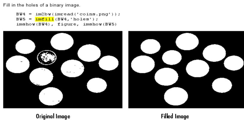
**Figure 2.7 Sample of filling holes**
